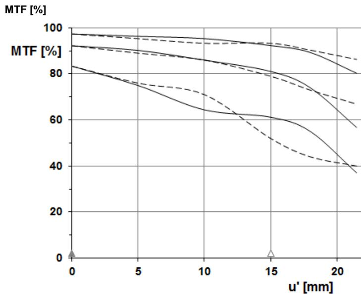
Modulation transfer MTF as a function of the image height ( $u'$ ) and slit orientation. White light. Spatial frequencies  $R=10, 20$  and  $40$  cycles/mm.
